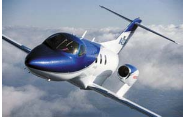
HondaJet's over-the-wing engine-mount reduces drag at high speed to improve fuel efficiency.
