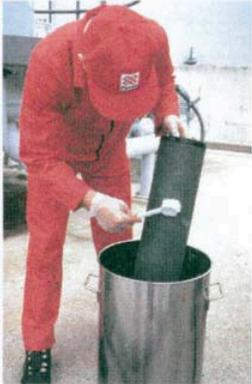
1. **CAREFULLY** remove each element from the filter separator.
