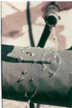
6. If the element passes the surface inspection (step 3) and the water test (step 5), rinse it thoroughly in clean fuel to remove traces of water and air dry prior to reinstalling.
