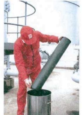
3. Allow excess fuel to run off. Holding the element by the endcaps, visually inspect the entire surface of the screen for damage and contamination. If there are any visible flaws or debris that have not been removed by washing, the cartridge should be replaced.
