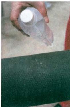
8. If there are visible tears, nicks, or cuts, they can be repaired as long as they are not larger than 1/8" in diameter. Use clear fingernail polish to repair the area. After you have repaired the element, wet the element in fuel and repeat the water test (step 5).
