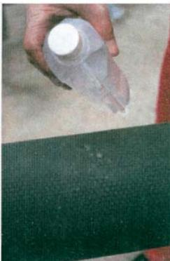
8. If there are visible tears, nicks, or cuts, they can be repaired as long as they are not larger than 1/8" in diameter. Use clear fingernail polish to repair the area. After you have repaired the element, wet the element in fuel and repeat the water test (step 5).
